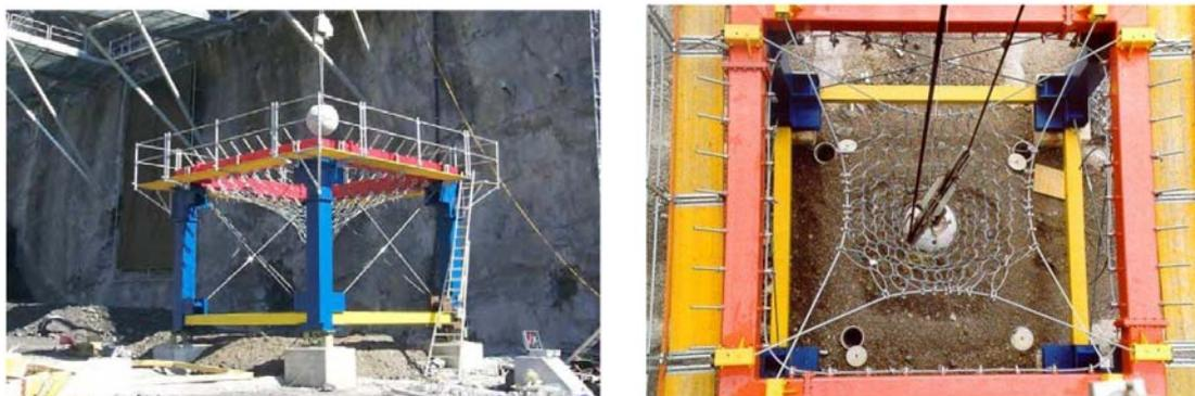
Plate 2: The specifically-built test rig for rock fall tests (Extracted from Volkwein, 2004)
